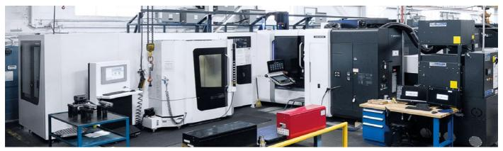
Included in Top Grade Molds' fleet of machines are four NHX 5000s, which operate automatically with two linear pallet pools.
