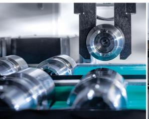
The gantry loaders handle workpieces into the respective machine, then remove and deposit the finished parts
