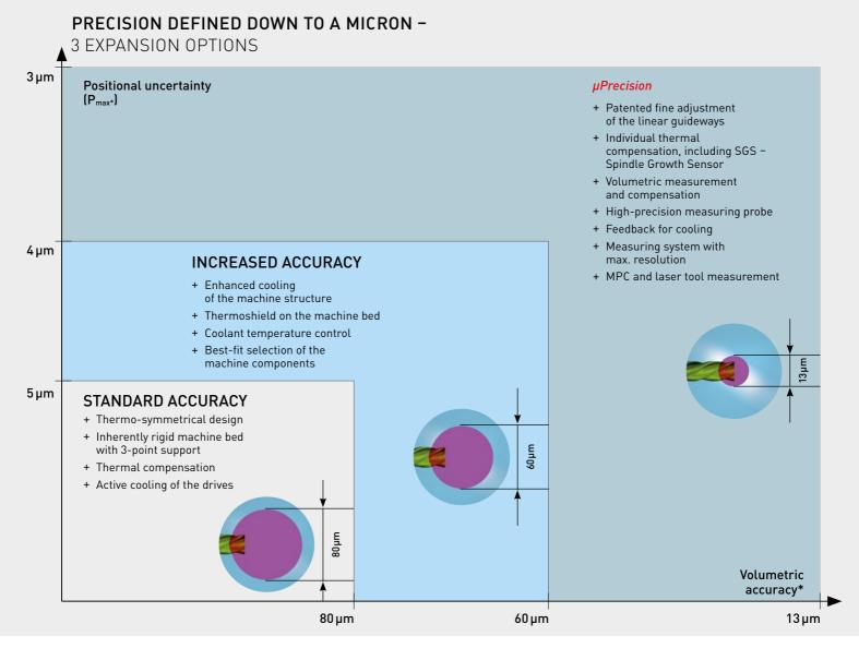
\*All values based on the DMU 80 P duoBLOCK //  $\mu$ Precision available for the duoBLOCK and Portal series (the specified installation and ambient conditions must be observed to achieve the accuracy values)
