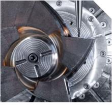
The original manufacturing process for complex impellers took as long as 25 weeks due to the production of the casting mold. Additive manufacturing on the LASERTEC 65 3D hybrid reduces this to less than a week
