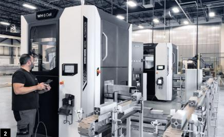
1. Automated manufacturing allows Attabotics to meet its high demand for base columns and other components, even at full capacity.  $\,$  2. The automated loading and unloading of the DMU 50  $3^{\rm rd}$  Generation achieves high production capacity and more manufacturing flexibility.
