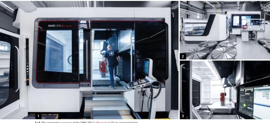
**1+2.** The volumetric accuracy of the DMU 210 U  $\mu Precision$  is 13  $\mu m$  and positioning accuracy is 4 µm in all axes. 3. A five-station pallet pool boosts the productivity of the DMU 210 U µPrecision.
