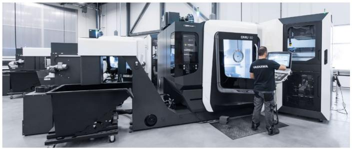
With automated production on the DMU 50 equipped with a WH 6 Cell, Attabotics meets the high demand for base columns and other components, even when at full production capacity.
