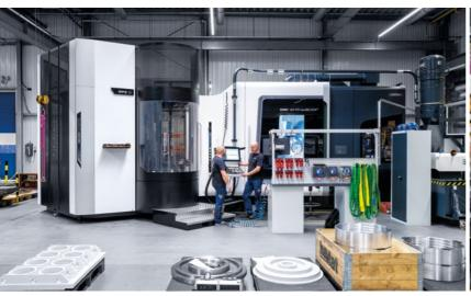
Equipped with grinding capability, the DMC 125 FD duoBLOCK achieves surface qualities down to 0.4  $\mu m$  Ra and circularity of 5  $\mu m$ .
