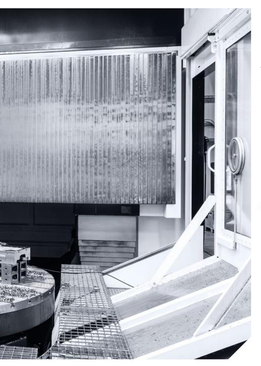
The work area of the DMU 340 P measures  $3,400 \times 3,400 \times 1,600$  mm. Maximum table load is 16 t.
