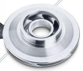
The ability to add material and mill workpieces alternately means that impellers can be manufactured with channels that run up to 360 degrees around the wheel.
